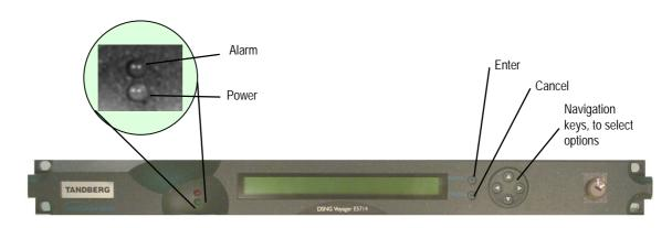
Figure 1.7: 1U Encoder Front Panel Indicators
